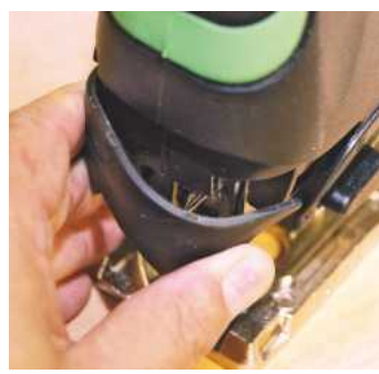
▲ The eject lever unlocks the clamp but you have to shake the blade loose
